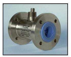
Our standard Teflon® turbines are supplied with PTFE for all wetted parts manufactured from blue-dyed Teflon® with the exception of the shaft which is normally manufactured from poly-ether-ether-ketone (PEEK) and the bearing and thrust washers which are a PEEK/PTFE blend. Please confirm PEEK is compatible with the intended service fluid. Other options are available.
